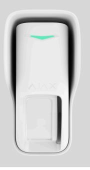
**Curtain Outdoor Jeweller** is a wireless curtain-type motion detector with dual motion detection technology for outdoor and indoor use. The detector has a horizontal detection angle of 8° and is designed for the perimeter control: windows, doorways, and other entrances or exits of the guarded facility. It detects motion at a distance of up to 12 m.
