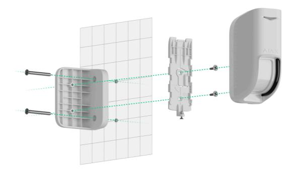
• **To a third-party mount**. The detector can be installed to a third-party mount with the SmartBracket mounting panel or hood.
