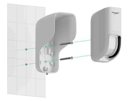
The hood replaces the detector's SmartBracket mounting panel, so you need to remove it before installing the detector with hood.
