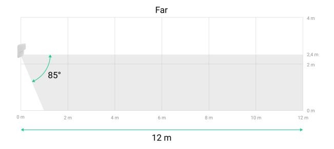
When choosing the installation site, consider the detector's horizontal viewing angle and the width of the detection zone. Incorrect placement of the detector may cause false alarms.
