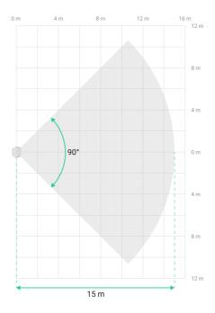
Horizontal characteristics of the motion detection area
