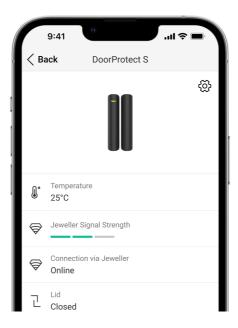
The states include information about the device and its operating parameters. The states of **DoorProtect S** can be found in the Ajax app:
