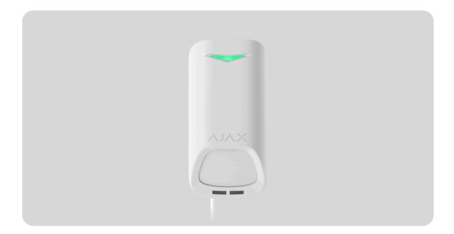
**Superior MotionProtect G3 Fibra** is a wired motion detector. It detects movement at a distance of up to 15 meters. In addition to using the IR sensor, the detector applies an additional radio frequency scan with a K-band microwave sensor that filters out infrared interference. Also, it features an anti-masking system that detects attempts to block the detector's field of view. The device is designed for indoor use only and complies with EN 50131 (Grade 3) requirements.
