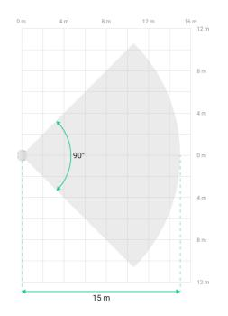
Horizontal characteristics of the motion detection area
