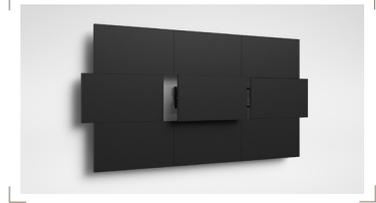
Slide one or several displays to the side for access: the selected display comes forwards to a service position 270 mm from the wall. This function makes it possible to service or exchange one display while the other displays remain in operation. You obtain full access to the sides and rear of the display to lay cables, service the display and achieve precise horizontal adjustment with the aid of a clever fine adjustment function at a minimum of 10 points.
