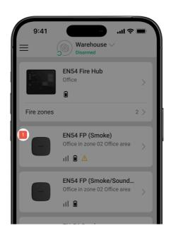
When an EN54 FireProtect (Smoke) Jeweller fault is detected, an Ajax app displays a fault counter on the device icon. All faults are indicated in the device states. Fields with faults are highlighted in yellow. Also, faults are displayed in the **Control** tab of the CIE display. More details about the fault can be found in the **Event center** or **Fire zones** tabs of the CIE.
