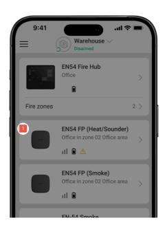
When an EN54 FireProtect (Heat/Sounder) Jeweller fault is detected, an Ajax app displays a fault counter on the device icon. All faults are indicated in the device states. Fields with faults are highlighted in yellow. Also, faults are displayed in the **Control** tab of the CIE display. More details about the fault can be found in the **Event center** or **Fire zones** tabs of the CIE.
