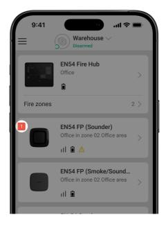
When an EN54 FireProtect (Sounder) Jeweller fault is detected, an Ajax app displays a fault counter on the device icon. All faults are indicated in the device states. Fields with faults are highlighted in yellow. Also, faults are displayed in the **Control** tab of the CIE display. More details about the fault can be found in the **Event center** or **Fire zones** tabs of the CIE.
