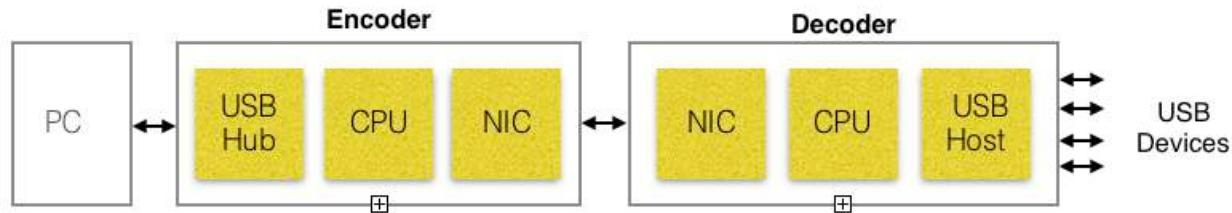
**Important Notes:** The Icron USB chipset requires its own independent IP address. This address can only be obtained via a DHCP server, or alternately it will take a Link-Local address.
