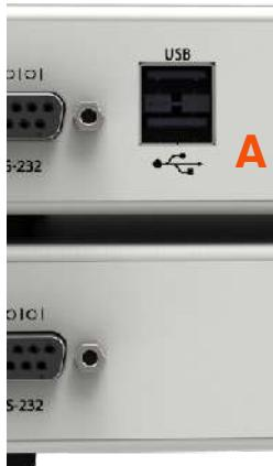
The ZyPer4K Decoder device can be ordered with optional USB connectivity.
