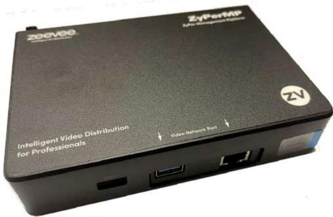
Most installations will require a ZyPer Management Platform (ZyPerMP). This device controls the operation and manages the connectivity between endpoints. The management platform is a hardened controller node that must reside on the same logical network as the ZyPer4K Encoders and Decoders. It runs a ZeeVee application as its sole function. The application presents an API to potential third party management platforms as well as hosting its own management application.
