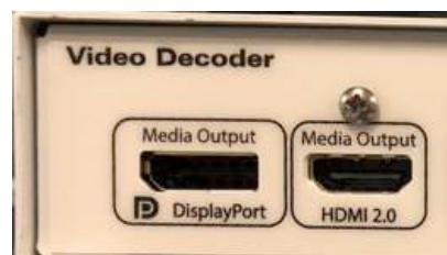
The ZyPer4K Decoder device can be ordered with an optional DisplayPort output.
