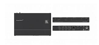
The FC-24ETH is an Ethernet control gateway, capable of plug and play deployment over a customer Ethernet LAN for remote control of customer controlled devices via bidirectional RS-232 or RS-485 serial control connections. Multiple control clients can be IP-connected to the FC-24ETH control gateway for concurrent control of two RS-232 or RS-485 controllable devices, such as AV scalers, video displays, and audio amplifiers.
