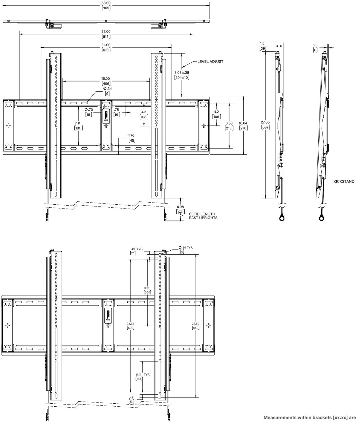
Measurements within brackets [xx.xx] are mm, measurements outside of brackets are inches.
