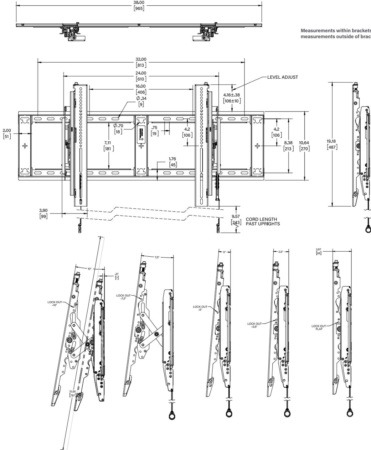
Measurements within brackets [xx.xx] are mm, measurements outside of brackets are inches.
