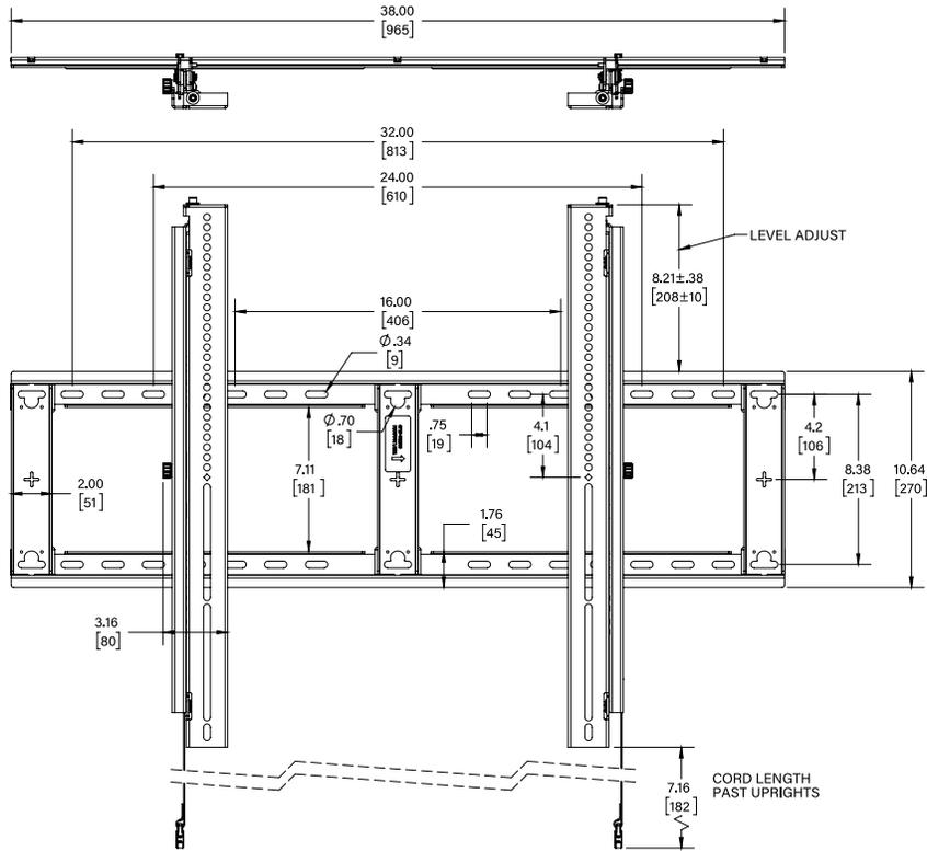
Measurements within brackets [xx.xx] are mm, measurements outside of brackets are inches.
