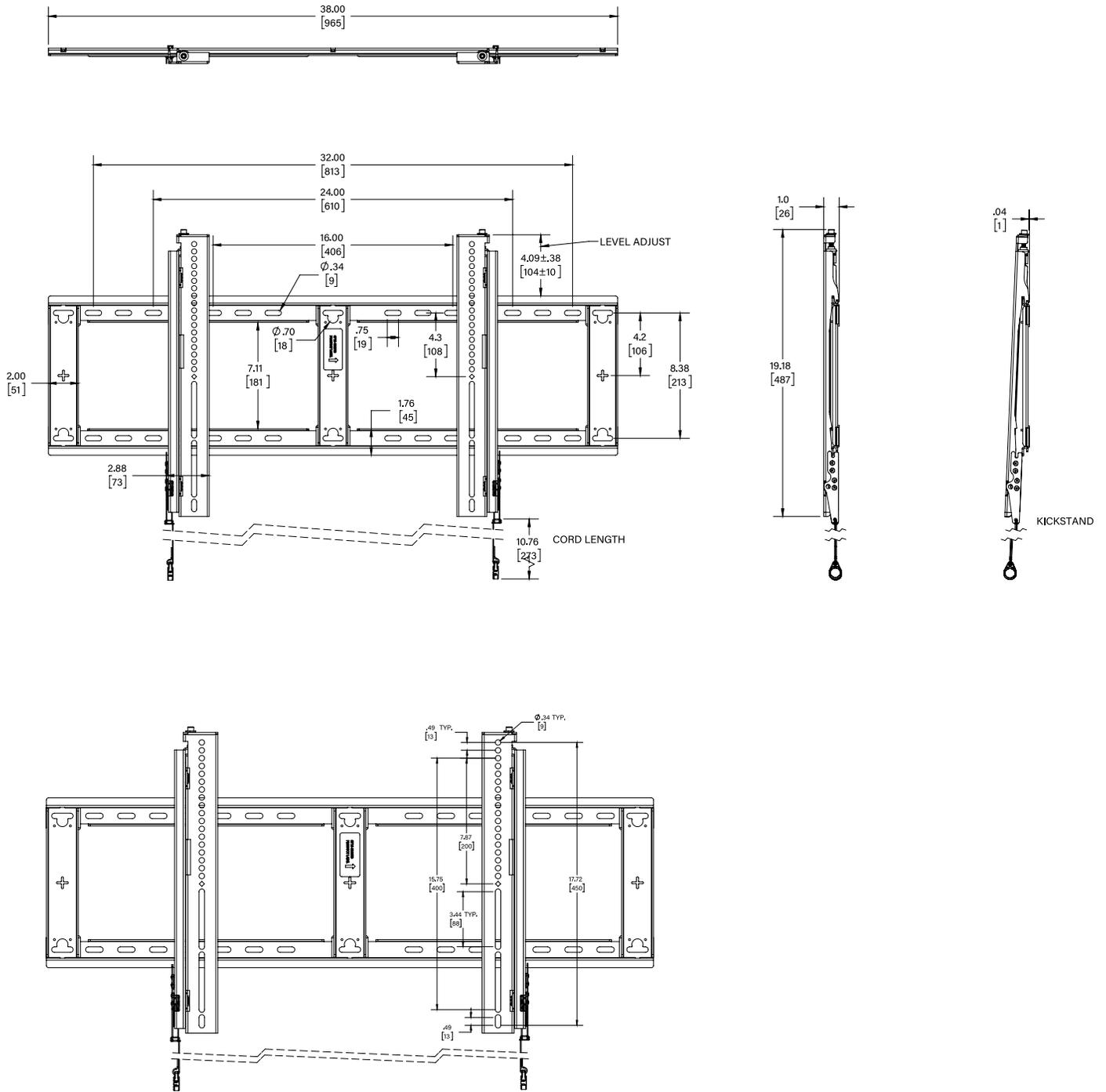
Measurements within brackets [xx.xx] are mm, measurements outside of brackets are inches.
