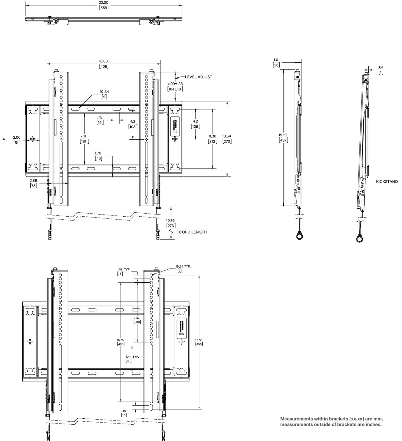
Measurements within brackets [xx.xx] are mm, measurements outside of brackets are inches.
