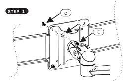
Mount the Dual bar. To an appropriate monitor arm. Lift the bar into position by aligning the VESA holes and pass the screws through one by one. If necessary use the washers and fasten using the nuts.
