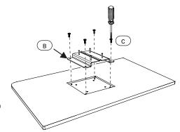
Place the LCD monitor face down on a flat surface. Align the VESA bracket holes and fasten using screws. Repeat procedure for both LCD monitors.
