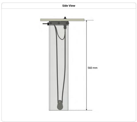
Detailed measurements for proper installation of the Ochno Pull Out Cable Management kit:
