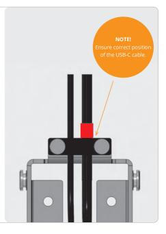
Step 16 Step 17 Secure the cables with screws.
