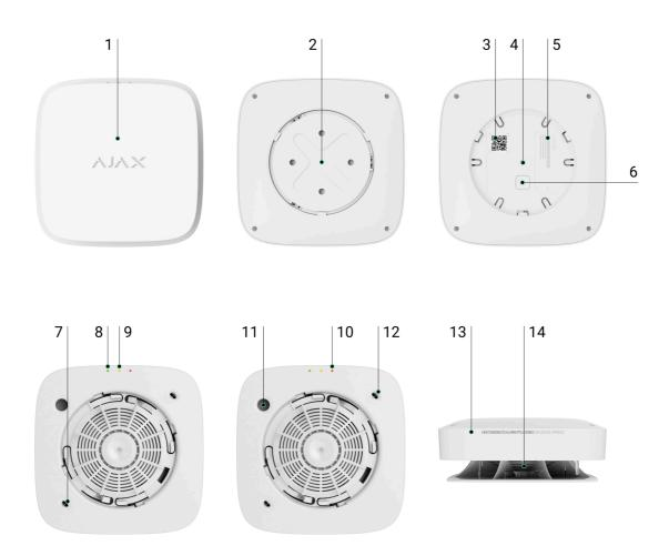
**1.** The front panel of the detector with a **Test/Mute button**. To activate the button, press the center of the panel.
