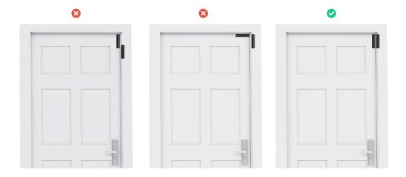
When mounting the detector on perpendicular planes, use a small magnet. The distance between the small magnet and the detector should not exceed 1 cm.
