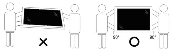
• Place the display vertically and its weight should spread evenly on the surface.
