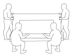
Carefully move the display until the bottom handles are out of the box. Two people on the sides should hold the 4 handles, while two others stand at the front and back of the display to support the bottom.
