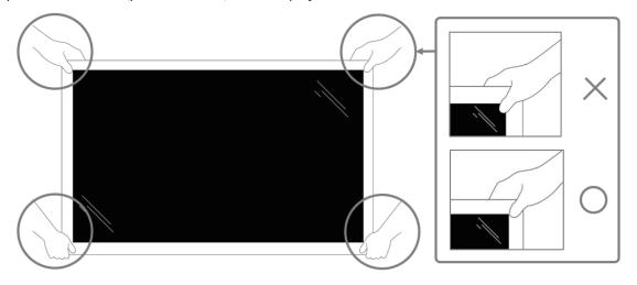
• When removing the display from the box, leave the protective bag inside and take care not to touch the glass of the display to avoid any damage.
