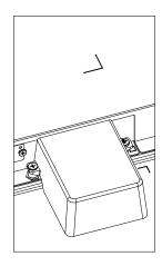
Maximum suitable size for the USB stick: USB: 20(W)x10(H)x60(L) mm
