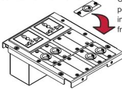
Carefully insert the power sockets and inserts to the inner frame.
