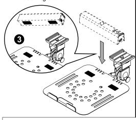
Take the elastic strap goes through two holes on the metal tray by stretching the strap carefully.
