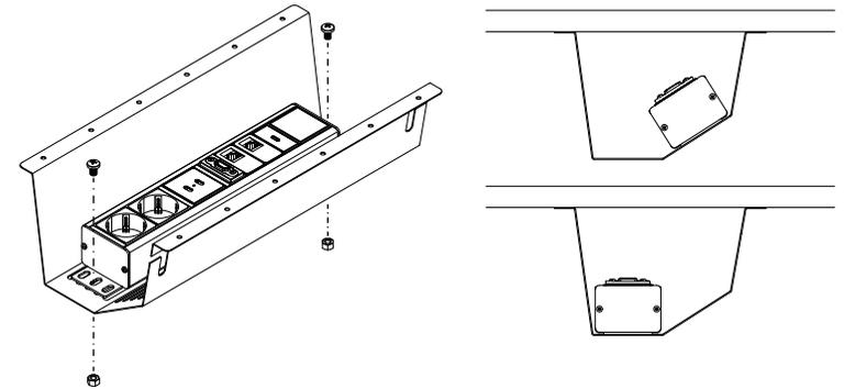
**2** Position tray under table and fixate with wood screws
