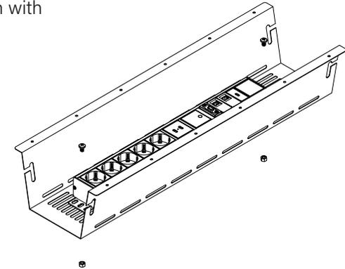
**2** Position tray under table and fixate with wood screws
