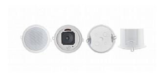
The Galil 2-C is a 2.5" full-range closed-back speaker with ceramic terminals and a plastic self-extinguishing back-can. It is especially designed to meet the requirements of fire alarm systems in public spaces and is EN 54-24 certified.
