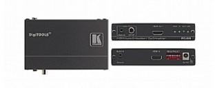
The FC-69 is a high-performance [email protected] (4:2:0) UHD, 4Kx2K HDMI audio embedder and de-embedder. The unit can embed analog audio to the HDMI output or de-embed audio from the HDMI input or from the HDMI output Audio Return Channel to S/PDIF and unbalanced stereo audio outputs simultaneously.
